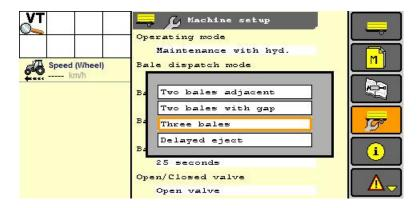
Please note that it is not possible to alter the bale dispatch program while there is a program in progress (i.e. there are bales on the deck). If that guideline is violated, the new selection shall be reverted to the previous one. In order to change a dispatch program, the operator must either wait until the program is finished (i.e. bale are ejected) or eject the bales manually.
