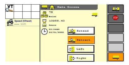
Pressing and holding down a button will move the respective bar to the desired direction.
