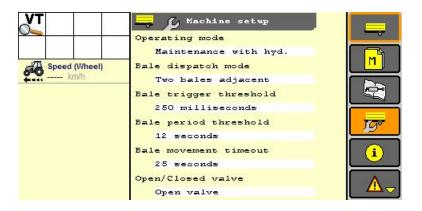
Selecting the "Operating Mode" field allows for the adjustment of the machine operating mode:
