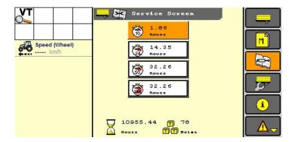
In order to confirm that maintenance has been carried out, select the indicated-by-red block and confirm:
