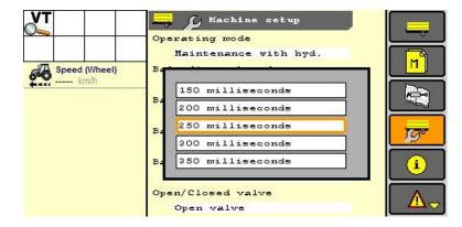
The "Bale Period Threshold" option determines the minimum time allowed between bales:
