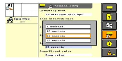
The Setting Open/Closed valve determines whether the system will control the center open valve as well as the hydraulic output (open valve) or only the output (closed valve).
