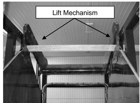
Note: Place board through safety block holder to block loader arm from falling unexpectedly.
