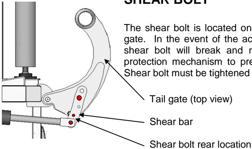
The shear bolt is located on the bottom of the hinge, on the gate. In the event of the accumulator being overloaded, the shear bolt will break and need to be replaced. This is a protection mechanism to prevent other parts from breaking. Shear bolt must be tightened to 220 lb-ft (n-m).
