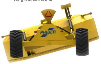
Blade relief allows dirt to roll, reducing HP Robust frame design, up to 75% stronger than competitive units
