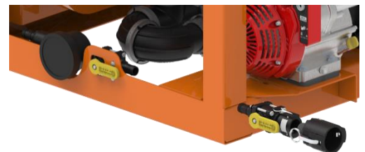
Figure 4.4- Aux. Chemical Meter
